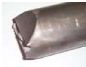
Normal "Pinch" Cut
